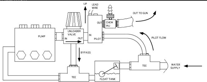
Install the flow switch *vertically* to the output side of the unloader, with the 2 conductor lead wires exiting from the top. If your system uses a downstream chemical injector, it should be mounted on the output side of the flow switch.
