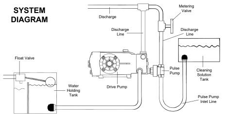
Pulse Pump will not draw cleaning solution with a pressurized inlet to the drive pump. For optimum performance inlet pressure to the drive pump should be zero or negative but not to exceed drive pump specifications.
