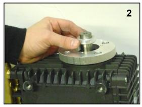
2. Install spacer ring on shaft.
