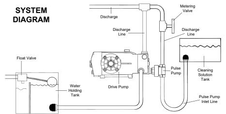
Pulse Pump will not draw cleaning solution with a pressurized inlet to the drive pump. For optimum performance inlet pressure to the drive pump should be zero or negative but not to exceed drive pump specifications.
