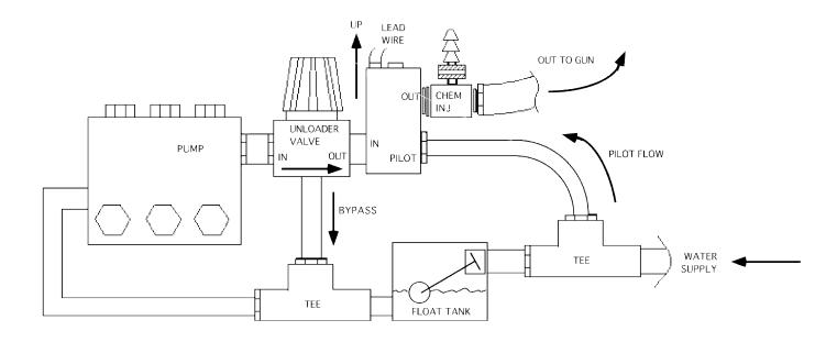
NOTE: When using this flow switch in a system containing a positive displacement pump, General Pump recommends the use of a safety relief device(s), correctly placed to protect all areas of the system.
