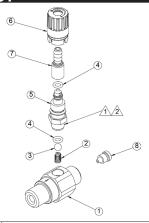
Apply Loc-tite® 545 to threads for re-assembly
