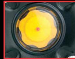
Large diameter of sight glass means easier oil checking
