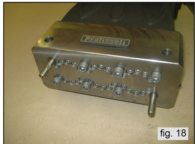
Unscrew the M10 x 210 head fixing screws No. 1 and No. 2 as shown in fig. 17 replacing them with two service pinscrews (#F27840000) as shown in fig. 18. Then take out the remaining screws.
