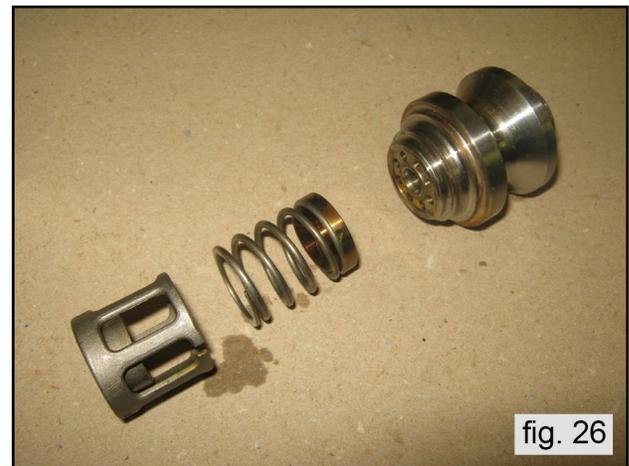
Extract the valve seat (1, fig. 25) check the various components for wear and replace them if necessary, see fig. 26.
