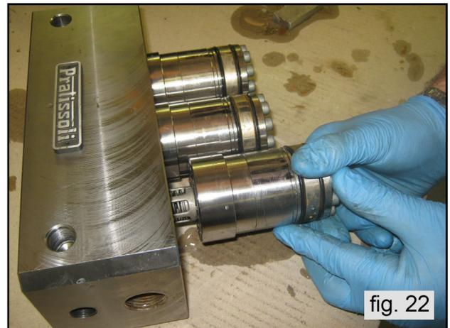
Take out the m6 x 75 screws fastening the liners to the head as shown in fig. 21 and proceed as shown in fig. 22.
