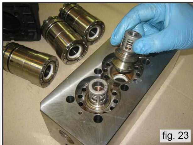
Remove the complete valve assemblies as indicated in fig. 23
