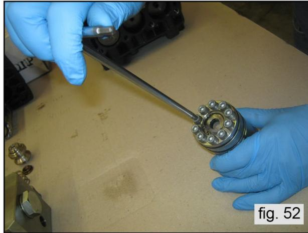
Assemble the L.P. and H.P. seals support units. Liner manually screwing the screws M6 x 65 as indicated in fig. 52. Then proceed with calibration using a torque wrench as indicated in chapter 3.
