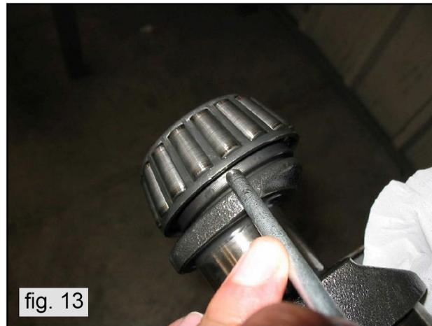
The new bearings can be mounted cold with a press or rocker, supporting it on the lateral surface of the ring nuts involved in press fitting with the rings. The press fitting operation can be assisted by heating the involved parts to a temperature between 250°F - 300°F (120°C - 150°C), ensuring that the ring nuts fit fully into their seats.
