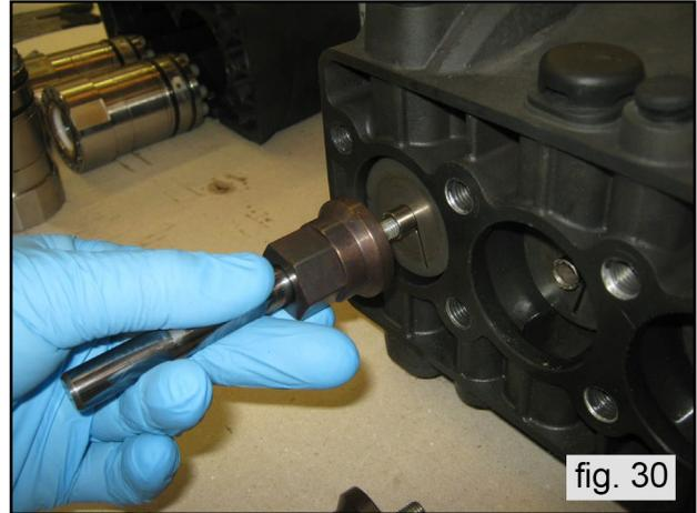
Remove the pumping element with a fork wrench and check for wear as indicated in fig. 29 and fig. 30, replace them if necessary.
