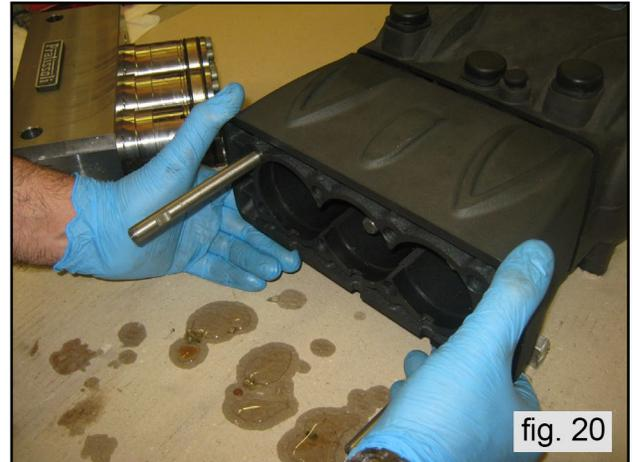
Separate the head and the spacer for the liners from the crankcase as shown in fig. 19 and fig. 20.
