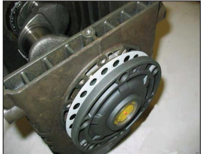
E) Insert the shims under the cover on the sight glass side (see fig. 11), fixing it to the crankcase using the appropriate screws, and verifying that the stall torque is between 3-4 ft. lbs. (4-6 Nm).
