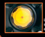
Large diameter of Oil dipstick with breather sight glass means easier oil checking
