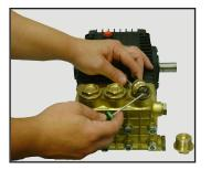
3) Remove plug to spacer O-ring.
