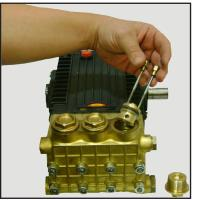
2) Remove outlet valve assembly from plug.
