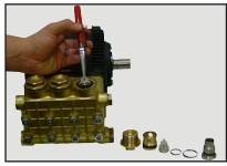
6) Remove lower spacer using 12 mm by 1.75 mm threaded bolt.
