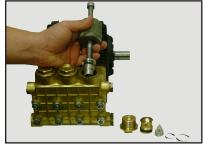
5) Remove inlet valve assembly.
