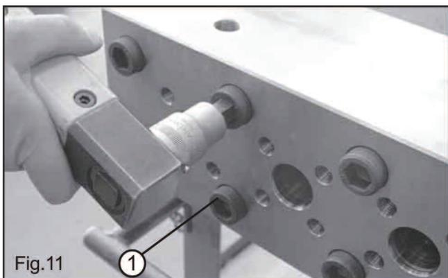
Loosen and remove the 8 head screws (1, Fig. 11).
