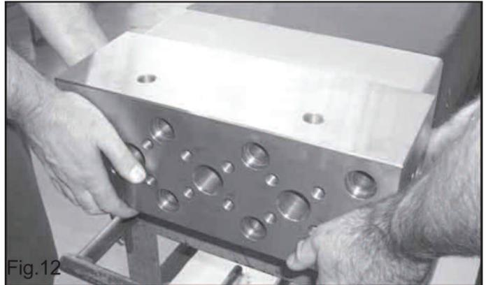
Remove the pump head (1, Fig. 12).
