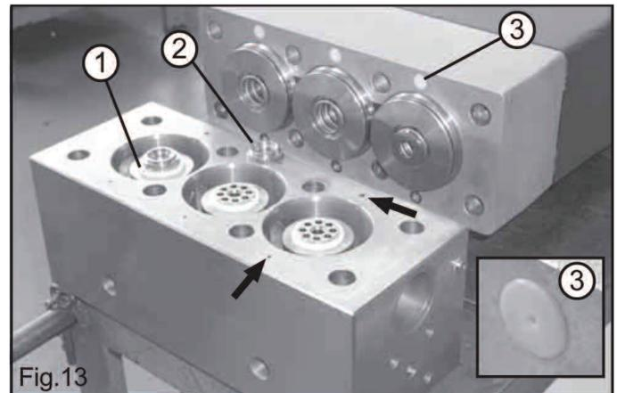
When removing the head from the pump pay attention to the valve seats (1, Fig 13) and the suction valve poppets (2, Fig. 13) which may fall off the head. Check the cooling system orifices of the head (see arrows) and the relevant white tips (3, Fig. 3) for deposits or sediments that may prevent cooling water from flowing through.
