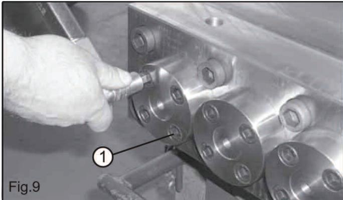
In order to have access to the delivery valves loosen the 12 valve cover screws (1, Fig. 9) and remove the covers.
