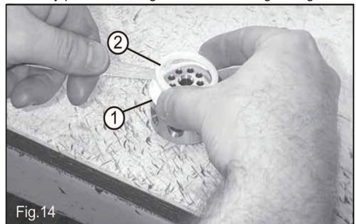
Remove the valve seats (1, Fig. 14) from the head, check them for wear and replace if necessary.
