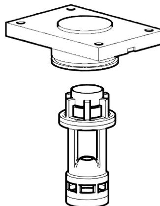
Valve components of each valve unit are pressed together in one single block and therefore they can be easily replaced and installed back in place. Separating the various components of the valve unit is carried out by means of simple tools as shown in Fig. 11, 12, 13 on page 11).
