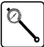
Reassemble the valve units and fit them back in the fluid end. Valve cover screws should be tightened with a torque wrench set for 86.7 ft. lbs.
