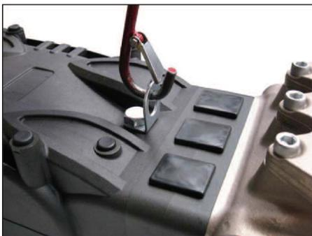
In case of disassembly, to avoid letting dirt inside the front part of the crankcase, close the threaded hole with the supplied cap.
