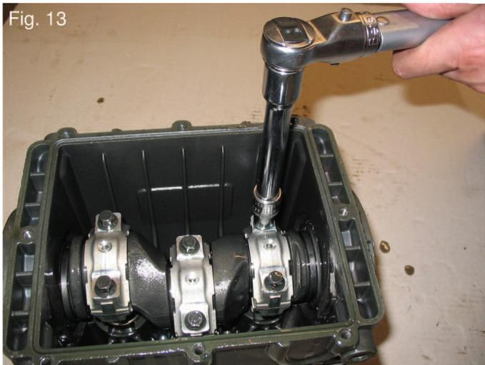
Note: The screws must be greased on the thread and under the head
