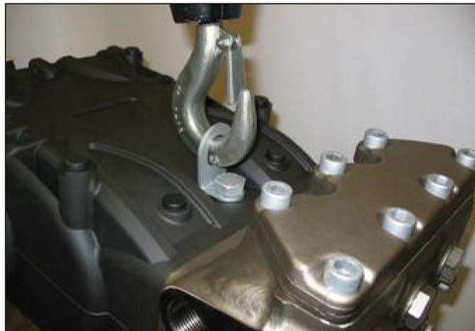
In case of disassembly, to avoid allowing debris inside the front part of the crankcase, close the threaded hole with the threaded cap.
