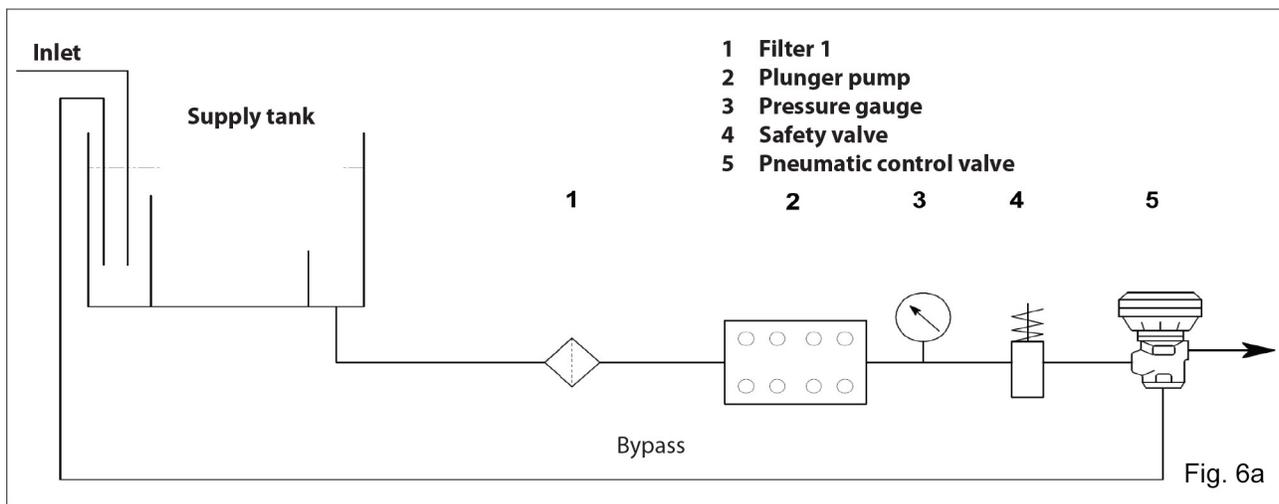
The filter must be installed as close as possible to the pump, should allow easy inspection and have the following characteristics:
