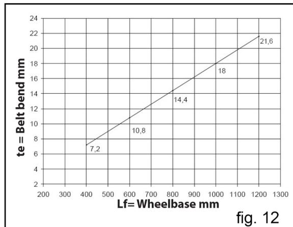
Conclusion: with a wheelbase of 23.62 in. (600 mm) and with a dynamometer, loading the belt branch with 16.86 lbs (75 N) as indicated in fig. 13 a “te” bend of approximately .43 in (10.8 mm) is obtained.
