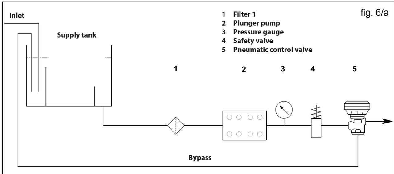
The filter must be installed as close as possible to the pump, should allow easy inspection and have the following characteristics:
