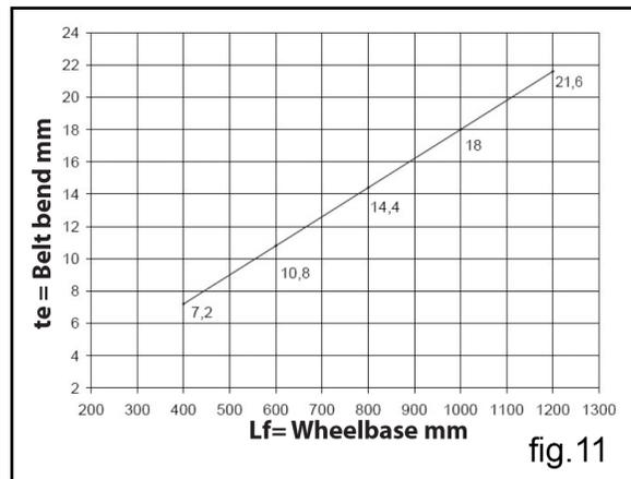
Conclusion: with a wheelbase of 23.62 in (600 mm) and with a dynamometer, loading the belt branch with 16.86 lbs (75 N) as indicated in fig. 12 a “te” bend of approximately .43 in (10.8 mm) is obtained.
