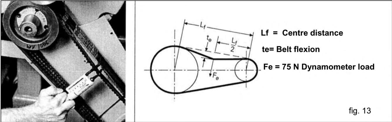
**Note 1:** If not differently indicated by the belt Manufacturer, the inspection of the correct tension value, and the related tension adjustment if needed is to be carried out after at least 30 minutes of operation in order to obtain belt setting. The best efficiency and maximum belt life is obtained with the correct tension value.
