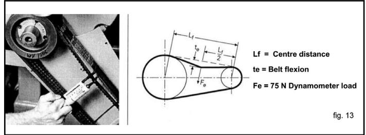
Note: If not differently indicated by the belt manufacturer, the inspection of the correct tension value, and the related tension adjustment if needed, is to be carried out after at least 30 minutes of operation in order to obtain belt settling. The best efficiency and maximum duration is obtained with a correct tension value.
