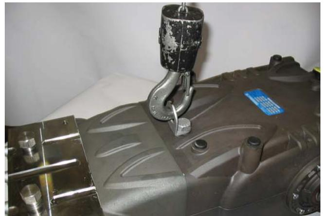
In case of disassembly, to avoid letting dirt inside the front part of the crankcase, close the threaded hole with the appropriate cap, supplied.
