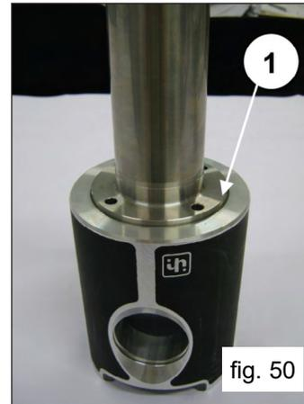
Place the stem in a vice, closing the teeth of the vice on the two flat areas, and proceed with setting, using a torque wrench (1, fig. 51) as shown in section 3.
