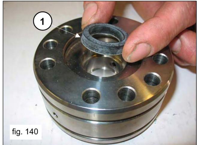
Reassemble the seal support assembly (1, fig. 141 and 142), replacing the 1, 2 and 3 components).
