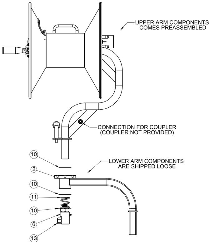
1. Slide washer (Item 10) over the shaft of the upper arm assembly.
