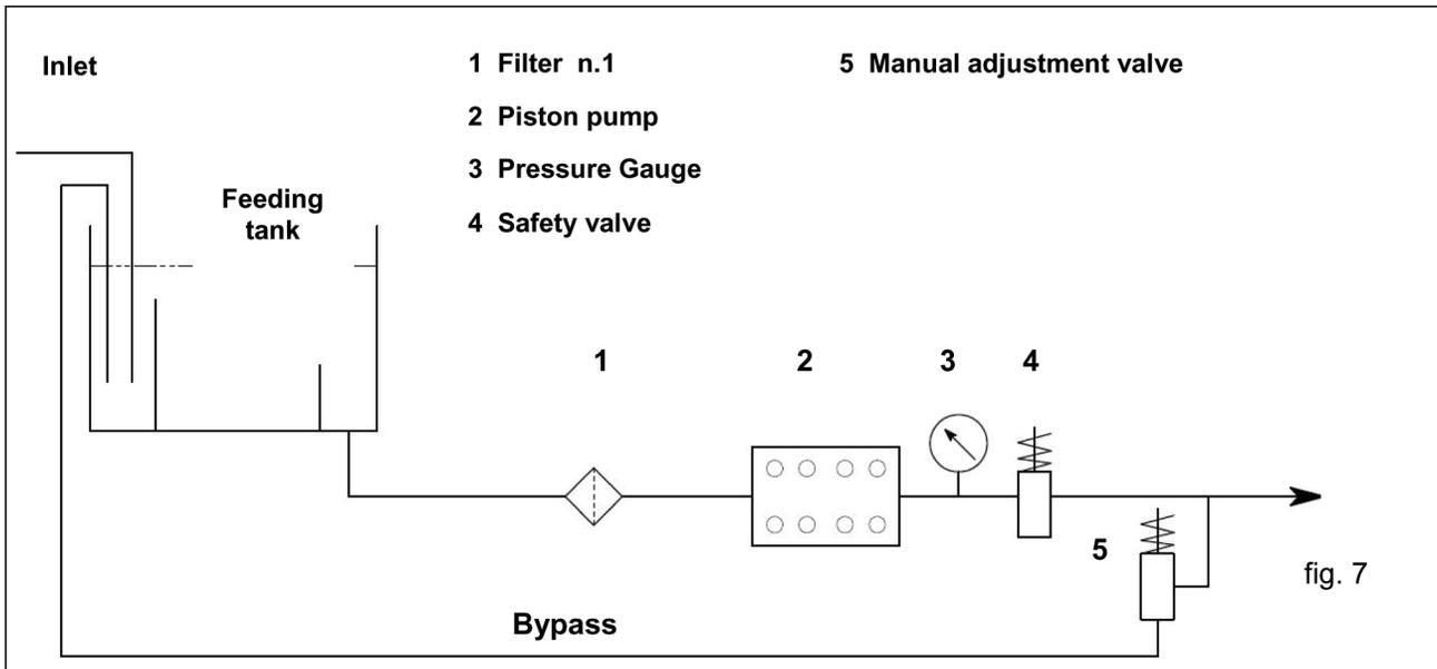
**Typical installation with hot water 95° F to 185° F (35° C to 85° C)**
