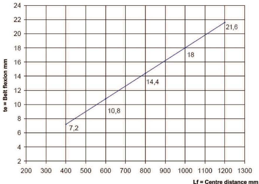
Finally, given a distance between pulley centers of 23.6 inches (600 mm) and a load of 75 N at the middle of the distance, a belt flexion “te” of around .425 inch (10.8 mm) will confirm the correct belt tension as shown in **fig. 13**.
