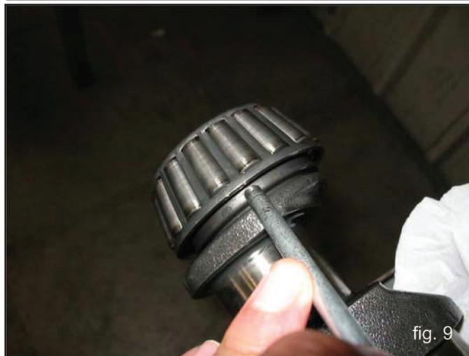
The new roller bearing can be mounted at room temperature with a press or fly press; it is necessary to lay them on the lateral side of the relevant ring nuts with correct rings. The driving operation can be facilitated by heating the relevant parts at a temperature ranging between 250°-300°F (120°-150°C), making sure that the ring nuts are correctly fitted into their seats.
