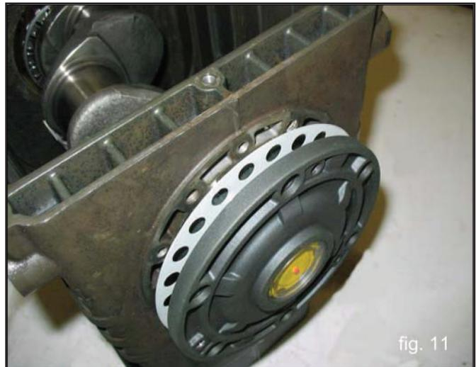
E) Insert the shims under the cover on the sight glass side (see fig. 11), fixing it to the crankcase using the appropriate screws, and verifying that the stall torque is between 3-5 ft. lbs. (4-7 Nm).
