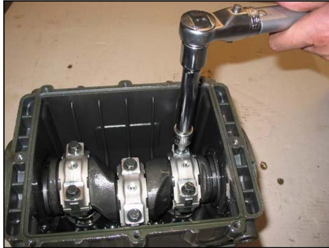
E) After setting the torque, check that the big end of the connecting rod has a lateral play in both directions.
