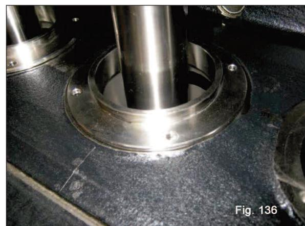
Tighten the (4) M6 screws (1, fig. 137) using a torque wrench, calibrating as described in Section 3.
