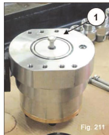
Lift the complete support and insert it into the front casing behind the manifold, after positioning the piston guide rod at bottom dead center (fig. 212), then fix the piston to the rod (1, fig. 213), tightening the screw with a torque wrench as described in Section 3.
