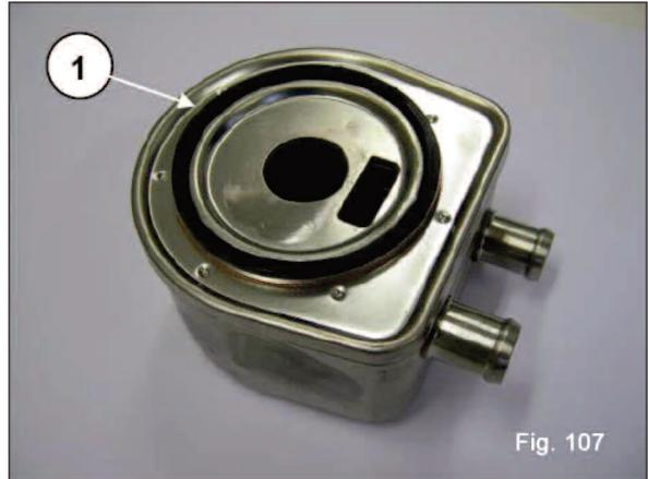
Fit the water-oil heat exchanger (1, fig. 108) and tighten the union with a torque wrench (1, fig. 109) as described in Section 3.
