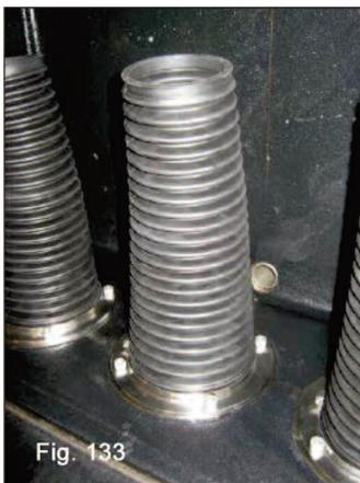
Remove the bellows and undo the (4) M6 fixing screws of the three bellows flanges (1, fig. 134).
