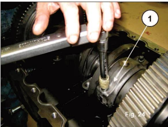
Remove the conrod caps with the bearing shells, taking special care to note the sequence in which they are removed.
