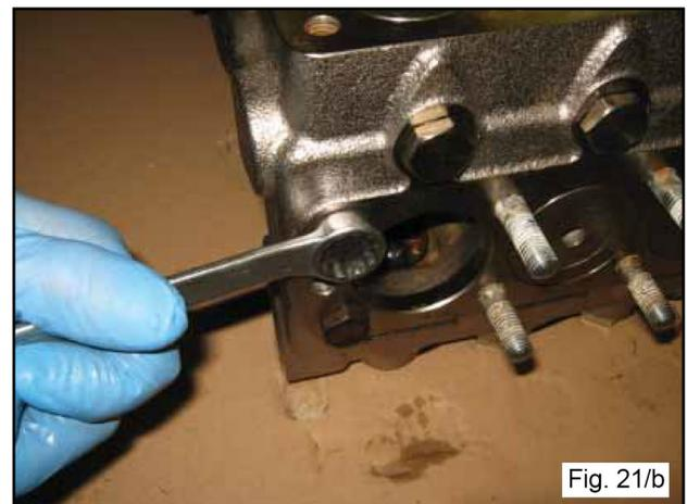
B) Remove the head and the head spacer from the pump casting.
