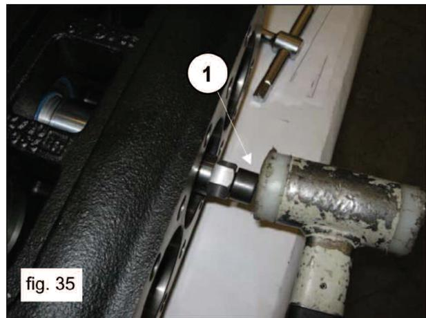
Extract the seal ring using the tool extractor hammer (1, fig. 36).
