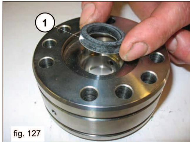
Reassemble the seal support assembly (1, fig. 128 and 129), replacing the 1 and 2 components).
