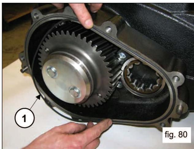
Complete assembly of the pinion on the reduction gear cover, proceeding as follows:
