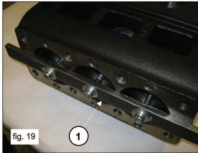
Remove the three upper half bearings of the half supports (1, fig. 20).
