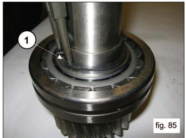
Insert the pinion preassembled inside its housing in the reduction gear cover, with the aid of an extractor hammer (1, fig. 86).
