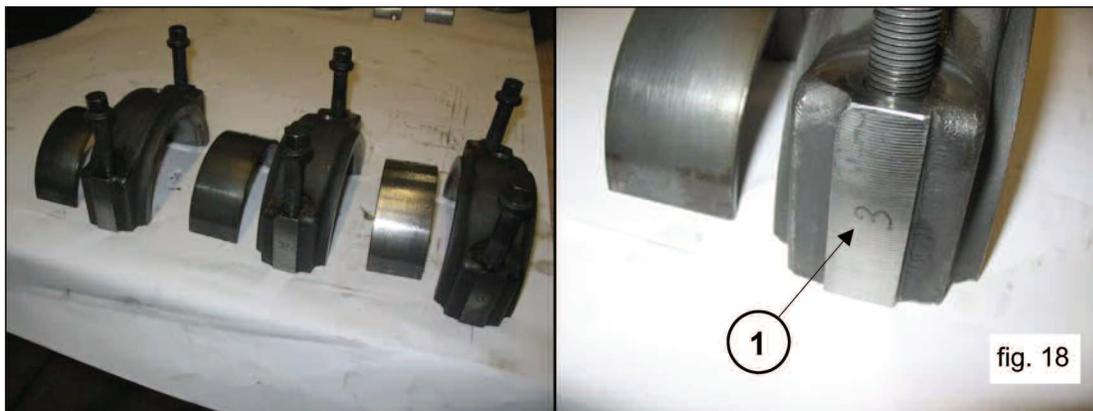
Advance the half supports completely in the direction of the hydraulic part to allow the crankshaft to come out. To facilitate this operation, use special too part #F27566200 (1, fig. 19).
