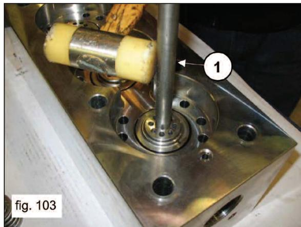
Extract the valve housings and check the conditions of the various components. If necessary, make any replacements (1, fig. 104).
