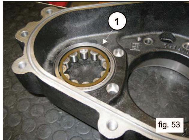
From the opposite side of the reduction gear box, preassemble the external ring of the crankshaft bearing with the use of tool part #F27605000 (1, fig. 54), inserting fully down to end stroke (1, fig. 55).
