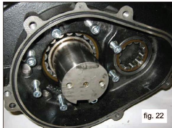
Position the 3 grub screws or M8 threaded screws (1, fig. 23) with the function of extractors in the holes and two sufficiently long M10 screws with the function of supporting the reduction gear box (2, fig. 23).
