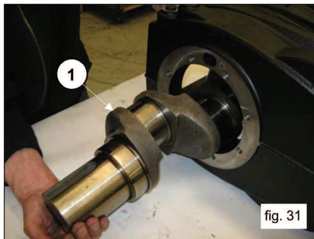
In the event that it is necessary to replace one or more connecting rods or plunger guides, operate as follows: unscrew the screws with tool part #F27566200 to unlock the connecting rods (1, fig. 32) and then extract the connecting rod/plunger guide units from the back casing opening (1, fig. 33).
