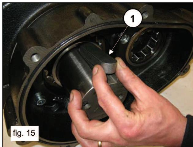
Remove the ring gear support ring (1, fig. 16).
