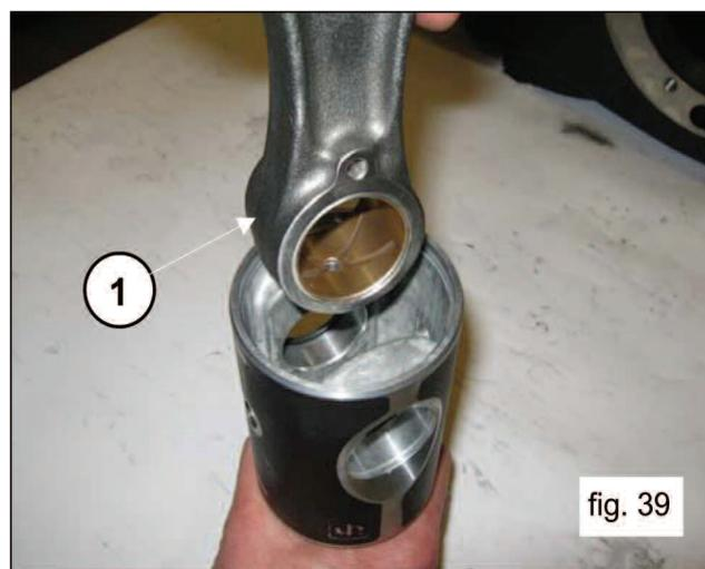
Couple the half supports to the previously disassembled caps, referring to the numbering (1, fig. 40).
