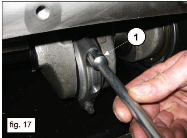
Remove the connecting rod caps with the lower semi-bearings, taking special care of the disassembly sequence during disassembly.
