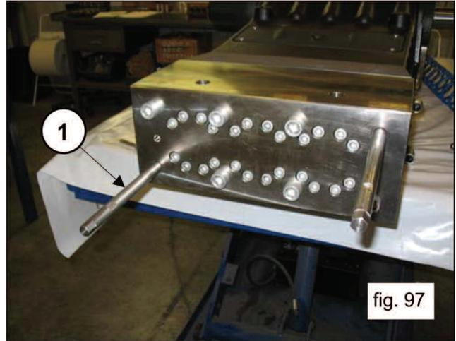
Separate the head and the spacer from the pump casing liners (1 fig. 98).
