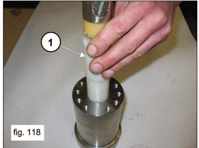
Insert the high pressure packing (1, fig. 119). Given the slight interference between the seal and the liner, use special tool part #F27673200 for SM14, SM16, and SM18, and part #F27673300 for SM20, SM22 and SM24 to prevent damage.
