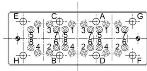
**Operation 1: M16x320 screw tightening , (pos. 1) in 2 phases**
