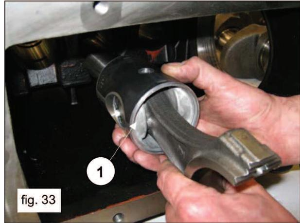
It is now possible to disassemble the plunger guide seal rings, taking care to not damage the plunger guide sliding rod.
