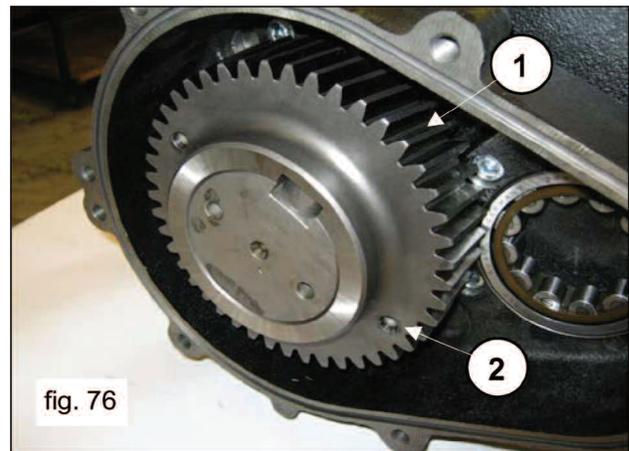
Fasten the ring gear stop (1, fig. 77) using (2) M10x25 screws. Calibrate the screws with a torque wrench as indicated in Section 3, "Screw Tightening Calibration" (1, fig 78).
