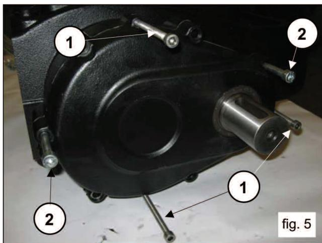
Slowly screw in the 3 M8 screws (1, fig. 6) with the function of extractors to fully remove the cover unit and pinion.
