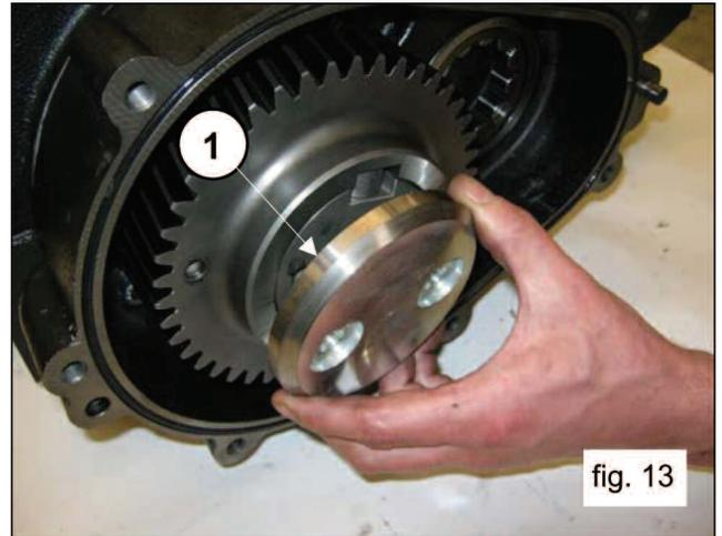
Remove the ring gear (1, fig. 14). Where necessary, it is possible to utilize an extractor hammer to be applied on the (2) M8 holes (2, fig. 14).
