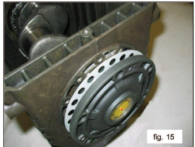
Once the type and number of shims have been determined using the table, check the following: assemble the shim pack on the indicator side cover centering (fig. 15). Secure the cover to the casing, following the procedure in part 2.1.2 and tighten the screws to their recommended torque.
