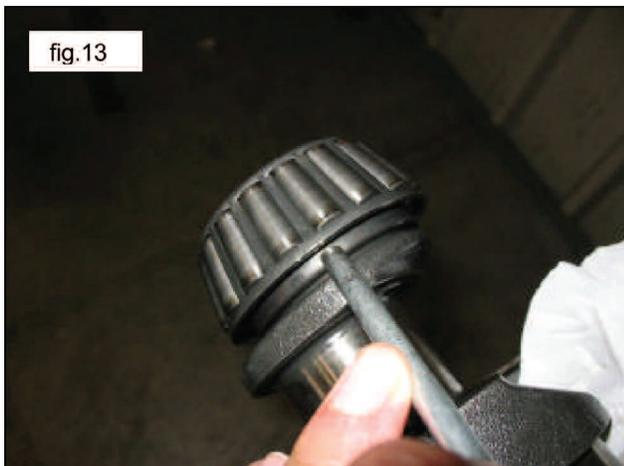
The new bearings can be mounted cold with a press or rocker, supporting it on the lateral surface of the ring nuts involved in press fitting with the rings. The press fitting operation can be facilitated by heating the involved parts to a temperature between 250°-300° F (120°-150° C), ensuring that the ring nuts go down to end stroke in their seats.
